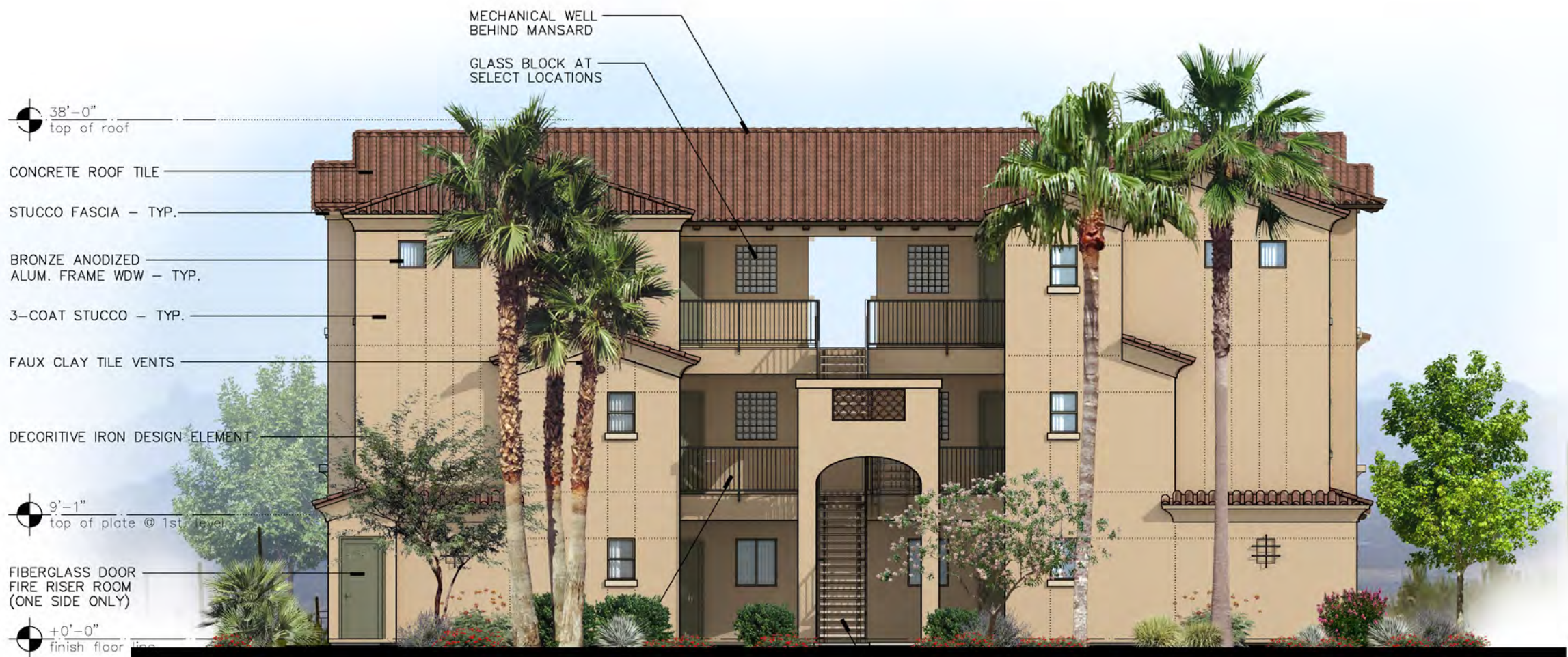
RIGHT ELEVATION (LEFT ELEVATION SIMILAR)
