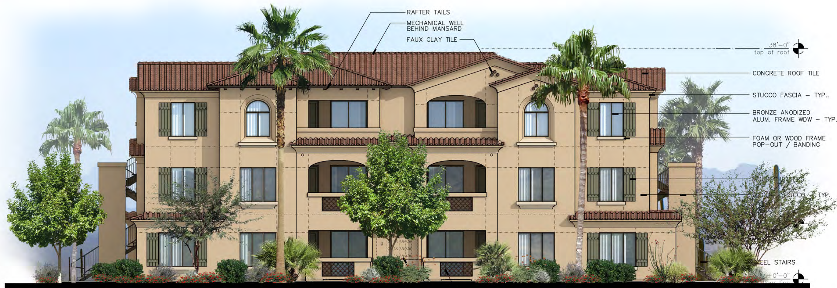
FRONT ELEVATION (REAR ELEVATION SIMILAR)
