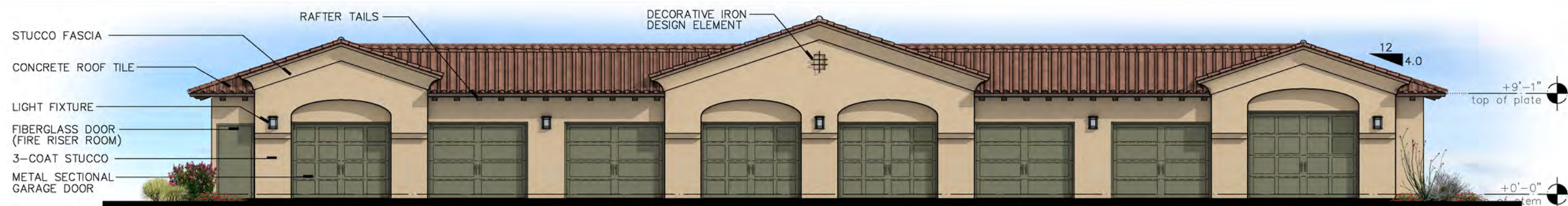
FRONT ELEVATION - GARAGE
